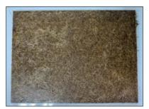
*Figure 2*. TPS/beeswax reinforced with coconut fiber
